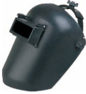
WM 008 Welding mask ,PP material, welding glasses size: 108*50*3mm thickness,welding glasses shade no.10(#7-14# for choice) ,flip design with open-close locking positioning. Whirl racket back.
