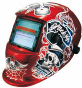
WM-A09 Auto-welding mask 1. Variable shade: DIN 9 -13. 2. Darkness adjustment: External. 3. Viewing area: 92*42mm. 4. Switching time of safety helmets shield: a) Light to dark: 1/25,000s. b) Dark to light: 0.1~1.0s, Steplessly adjustable. 5. Sensitivity:low to high, Steplessly adjustable. 6. Light state: shade DIN 4. 7. UV/IR protection: up to shade DIN 15 at all time. 8. Power on/off : Automatic. 9. Power supply: Large solar cells, two lithium batteries. 10. Mode: Weld /Grind. 11. Warranty: 2 years. 12. Material & Weight: PP, 0.48kgs. 13. Fire resistanc: yes. 14. Dimension: 360mm*240mm*230mm. 15. Operating Temperature: -10℃~+ 55℃. 16. Storage Temperature: -20℃~+70℃.
