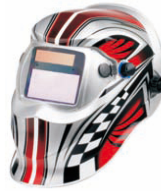
WM-A03 Auto-welding mask 1. Variable shade: DIN 9 -13. 2. Darkness adjustment: External. 3. Viewing area: 98*44mm. 4. Switching time of safety helmets shield: a) Light to dark: 1/25,000s. b) Dark to light: 0.1~1.0s, Steplessly adjustable. 5. Sensitivity:low to high, Steplessly adjustable. 6. Light state: shade DIN 4. 7. UV/IR protection: up to shade DIN 16 at all time. 8. Power on/off : Automatic. 9. Power supply: Large solar cells, two lithium batteries. 10. Mode: Weld /Grind. 11. Warranty: 2 years. 12. Material & Weight: PP, 0.48kgs. 13. Fire resistanc: yes. 14. Dimension: 360mm*240mm*230mm. 15. Operating Temperature: -10℃~+ 55℃. 16. Storage Temperature: -20℃~+70℃.
