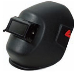
WM 010 Welding mask ,PP material, welding glasses size: 108*50*3mm thickness,welding glasses shade no.10(#7-14# for choice) ,flip design with open-close locking positioning. Whirl racket back.
