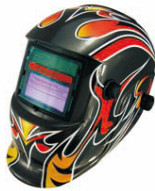
WM-A08 Auto-welding mask 1. Variable shade: DIN 9 -13. 2. Darkness adjustment: External. 3. Viewing area: 92*42mm. 4. Switching time of safety helmets shield: a) Light to dark: 1/25,000s. b) Dark to light: 0.1~1.0s, Steplessly adjustable. 5. Sensitivity:low to high, Steplessly adjustable. 6. Light state: shade DIN 4. 7. UV/IR protection: up to shade DIN 15 at all time.. 8. Power on/off : Automatic. 9. Power supply: Large solar cells, two lithium batteries. 10. Mode: Weld /Grind. 11. Warranty: 2 years. 12. Material & Weight: PP, 0.48kgs. 13. Fire resistanc: yes. 14. Dimension: 360mm*240mm*230mm. 15. Operating Temperature: -10℃~+ 55℃. 16. Storage Temperature: -20℃~+70℃.
