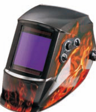
WM-A12 Auto-welding mask 1.Viewing Area: 101*94mm 2.Range of UV/IR protection: DIN 16 3.Light Shade: DIN 3 4.Dark Shade: DIN 5-9, 9-13, External control 5.Power on/off: Automatic 6.Switching Time (light to dark) : 1/30000s 7.Switching Time(dark to light): 0.1-1.0s, Steplesslyadjustable,External control 8.Sensitivity: Low to high, Steplessly adjustable,External control 9.Mode: Weld/Grind, External control 10.Arc sensor:4 11.Low Volume Alarm 12.ADF Self-check 13.Power Supply: Two solar cell and lithium batteries be changed 14.Operating Temperature: -10℃~+ 55℃. 15.Storage Temperature: -20℃~+70℃.
