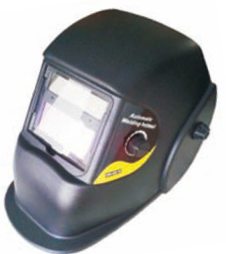
WM-A11 Auto-welding mask 1. Variable shade: DIN 9 -13. 2. Darkness adjustment: External. 3. Viewing area: 92*42mm. 4. Switching time of safety helmets shield: a) Light to dark: 1/25,000s. b) Dark to light: 0.2~0.4s, Steplessly adjustable. 5. Sensitivity:low to high, Steplessly adjustable. 6. Light state: shade DIN 4. 7. UV/IR protection: up to shade DIN 15 at all time. 8. Power on/off : Automatic. 9. Power supply: Large solar cells, two lithium batteries. 10. Mode: Weld /Grind. 11. Warranty: 2 years. 12. Material & Weight: PP, 0.48kgs. 13. Fire resistanc: yes. 14. Dimension: 360mm*240mm*230mm. 15. Operating Temperature: -10℃~+ 55℃. 16. Storage Temperature: -20℃~+70℃.
