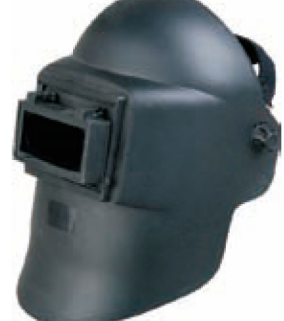
WM 004 Welding mask ,PP material, welding glasses size: 108*50*3mm thickness,welding glasses shade no.10(#7-14# for choice) ,flip design with open-close locking positioning. Whirl racket back.
