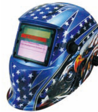
WM-A07 1. Variable shade: DIN 9 -13. 2. Darkness adjustment: External. 3. Viewing area: 92*42mm. 4. Switching time of safety helmets shield: a) Light to dark: 1/25,000s. b) Dark to light: 0.1~1.0s, Steplessly adjustable. 5. Sensitivity:low to high, Steplessly adjustable. 6. Light state: shade DIN 4. 7. UV/IR protection: up to shade DIN 15 at all time.. 8. Power on/off : Automatic. 9. Power supply: Large solar cells, two lithium batteries. 10. Mode: Weld /Grind. 11. Warranty: 2 years. 12. Material & Weight: PP, 0.48kgs. 13. Fire resistanc: yes. 14. Dimension: 360mm*240mm*230mm. 15. Operating Temperature: -10℃~+ 55℃. 16. Storage Temperature: -20℃~+70℃.
