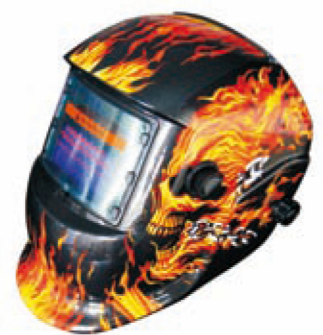
WM-A10 Auto-welding mask 1. Variable shade: DIN 9 -13. 2. Darkness adjustment: External. 3. Viewing area: 92*42mm. 4. Switching time of safety helmets shield: a) Light to dark: 1/25,000s. b) Dark to light: 0.1~1.0s, Steplessly adjustable. 5. Sensitivity:low to high, Steplessly adjustable. 6. Light state: shade DIN 4. 7. UV/IR protection: up to shade DIN 15 at all time. 8. Power on/off : Automatic. 9. Power supply: Large solar cells, two lithium batteries. 10. Mode: Weld /Grind. 11. Warranty: 2 years. 12. Material & Weight: PP, 0.48kgs. 13. Fire resistanc: yes. 14. Dimension: 360mm*240mm*230mm. 15. Operating Temperature: -10℃~+ 55℃. 16. Storage Temperature: -20℃~+70℃.
