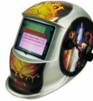
WM-A06 Auto-welding mask 1. Variable shade: DIN 9 -13. 2. Darkness adjustment: External. 3. Viewing area: 92*42mm. 4. Switching time of safety helmets shield: a) Light to dark: 1/25,000s. b) Dark to light: 0.1~1.0s, Steplessly adjustable. 5. Sensitivity:low to high, Steplessly adjustable. 6. Light state: shade DIN 4. 7. UV/IR protection: up to shade DIN 15 at all time. 8. Power on/off : Automatic. 9. Power supply: Large solar cells, two lithium batteries. 10. Mode: Weld /Grind. 11. Warranty: 2 years. 12. Material & Weight: PP, 0.48kgs. 13. Fire resistanc: yes. 14. Dimension: 360mm*240mm*230mm. 15. Operating Temperature: -10℃~+ 55℃. 16. Storage Temperature: -20℃~+70℃.
